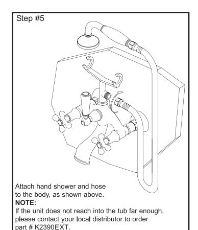
This kit will extend the unit 2" further into the tub.
